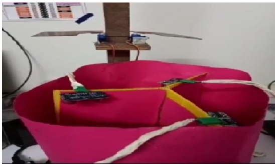
Fig 10: When the garbage gets detected and the flip gets open and the garbage falls in the following section.
